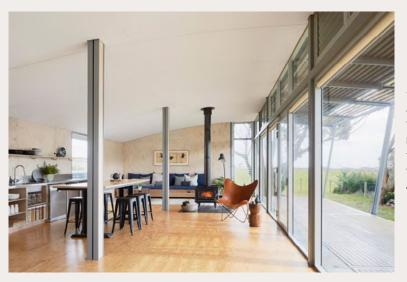
As part of the build, the tired internal plasterboard and floors were replaced with whitewashed and sealed plywood.
